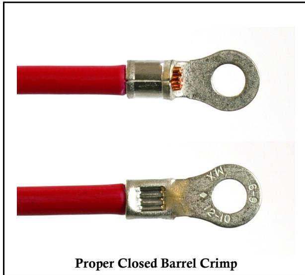
**Proper Closed Barrel Crimp**
