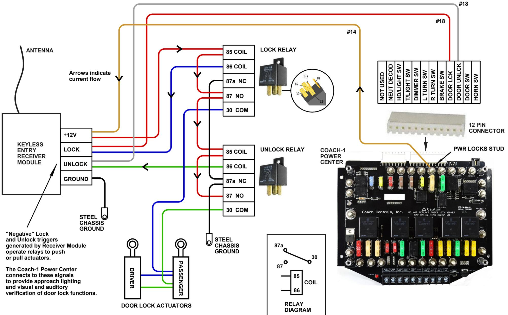
"Negative" Lock and Unlock triggers generated by Receiver Module operate relays to push or pull actuators.
