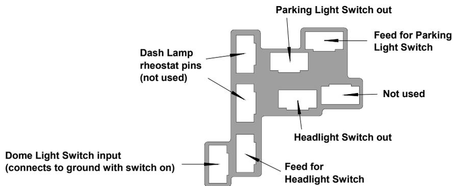
NOTE: The Headlight Switch does not carry any high currents, it simply triggers the Parking Lamp and Headlight relays on the Power Center.
