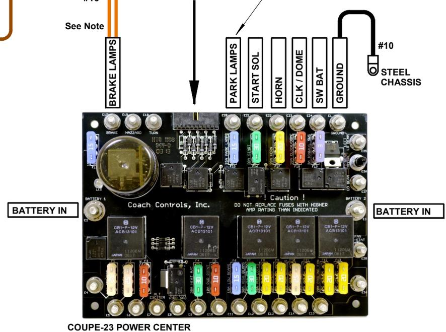
**NOTE:** In this configuration the Power Center Parking Light output terminal is not used at all. Instead, power from the Brake Switch terminal is used to supply power to the Rear Tail Lights, Front Parking Lights, and Dash Lights, all controlled by the Headlight Switch. The Brake Switch terminal also feeds power to the Brake Light circuit as shown on the complete system diagram.
